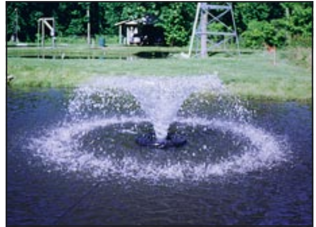
LEFT: Windmill connected to an air pump. BELOW: Fountain working as an aerator.
