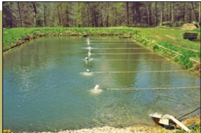
Group of diffusers held up off the bottom by one-gallon jugs. Air comes from a blower.
